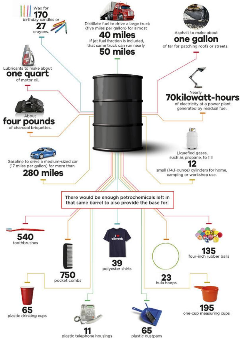
The lighter materials in a barrel are used mainly for paint thinners and dry-cleaning solvents, and they can make nearly a quart of one of these products. The miscellaneous fraction of what is left still contains enough byproducts to be used in medicinal oils, still gas, road oil and plant condensates.
